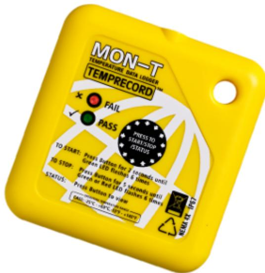
The Mon-T logger is a smaller form factor low-cost logger intended for mass deployment in produce shipping. Despite the smaller size it can still be inserted into the Temprecord Reader Interface and programmed and read.
