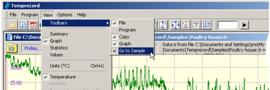
When you exit Temprecord, the position and state (docked or undocked) of each toolbar is saved. When you start Temprecord next, the toolbars are restored to their saved positions.
