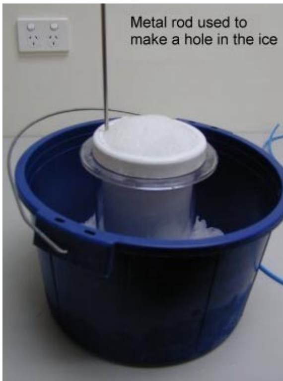
Making hole for syphon hose using 5mm-diameter metal rod.
